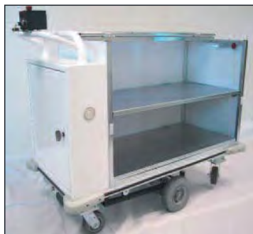
Custom Order Picking Carts Cart features flip up middle shelf for easy access to lower shelf.
