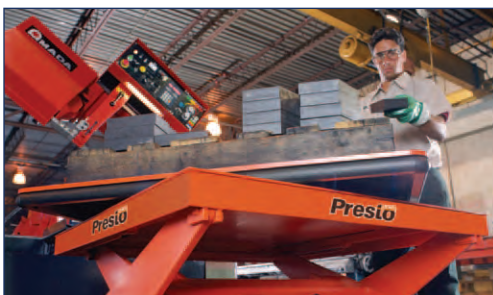
Standard Turntable shown mounted on Hydraulic Lift
