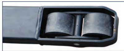
Tandem polyurethane load wheels
