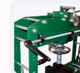
Hand Crank & Rotary Handle (positions the ram laterally)
