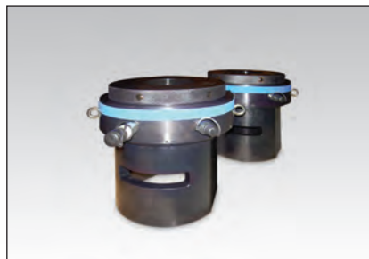
◀ Custom hydraulic tensioners to suit 5-inch studs load output 944202 lbf (4200 kN).
